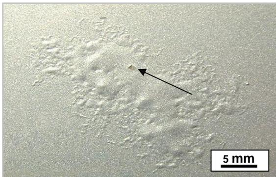
**Filiform corrosion** attack on aluminum part from a vehicle in service. The arrow points to the paint defect where the corrosion initiated.
