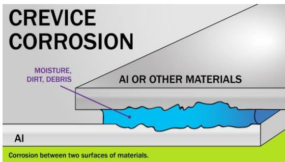
**Crevice corrosion** occurring between two materials. The mating surfaces can be aluminum to aluminum, aluminum to steel, or aluminum to plastic.
