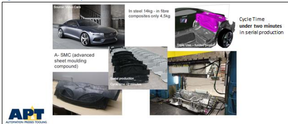
Figure 32: A-SMC Components Formed in Less than 2 Minutes
