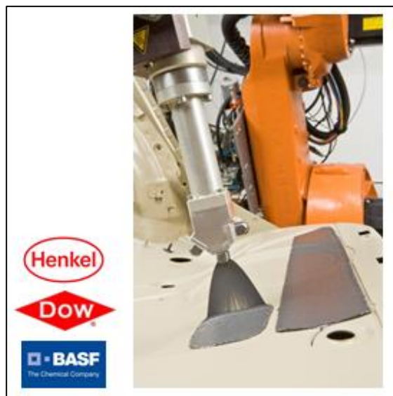
Figure 23: Automated Application of Liquid Applied Sound Deadener
