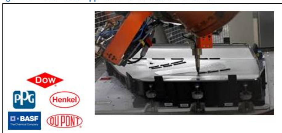
Figure 19: Automated Application of Structural Adhesives
