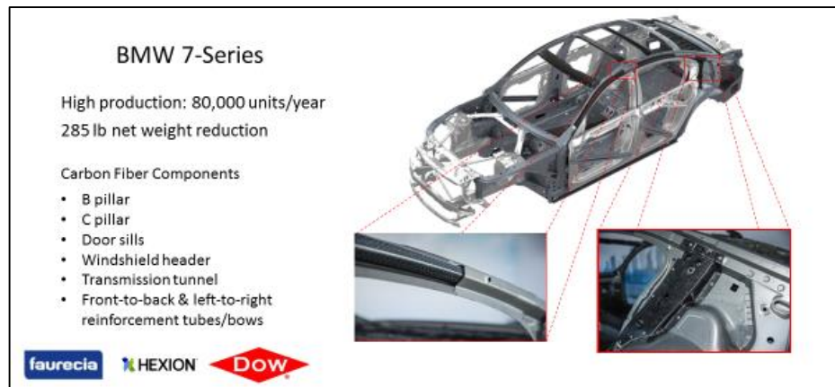
Figure 38: Carbon Fiber Application Expansion (BMW 7-Series)
