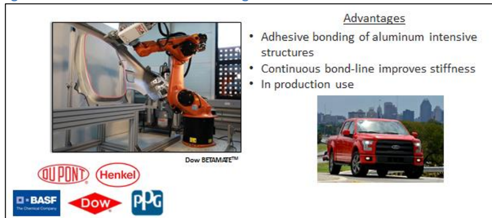
Figure 26: Structural Adhesives Enabling Mixed Materials
