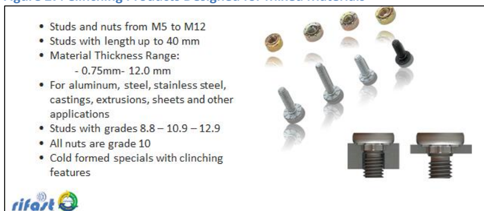
Figure 27: Clinching Products Designed for Mixed Materials
