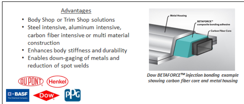
Figure 40: CFRP A-Pillar Insert Supported by Injected Structural Adhesive (Dow BETAFORCE™)
