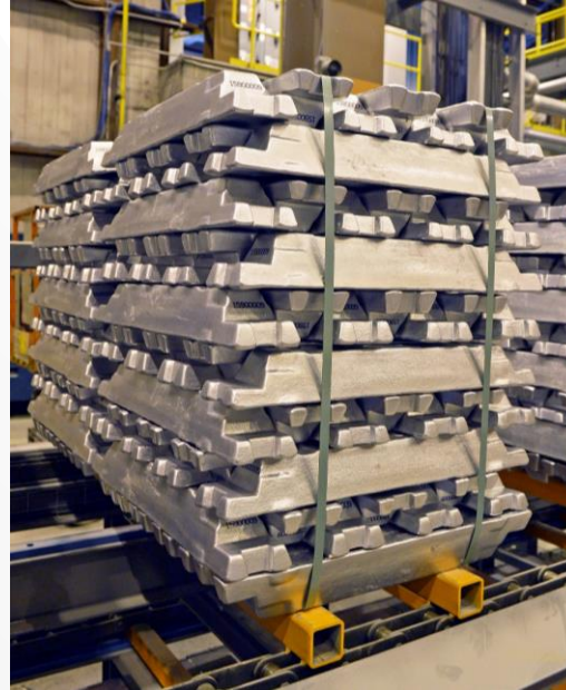
Small form cast ingot 6 to 23kg (15kg typical)
