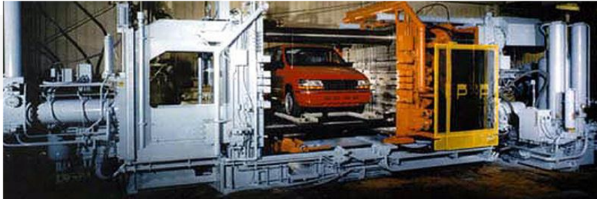
High pressure die casting (+ vacuum)
