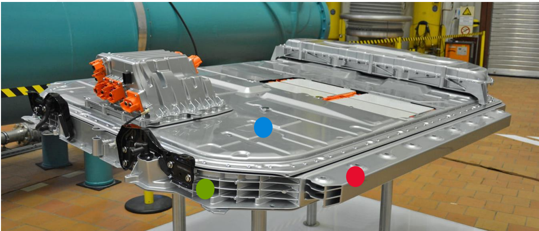
Large high-voltage battery (95 kWh of energy), around 700 kilograms (1,543.2lb)
