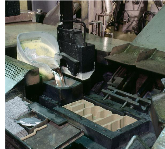
Gravity die casting: cylinder head, block (Rotocast®)
